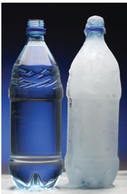
▲ FIGURE 11.12 Expansion of water upon freezing.
