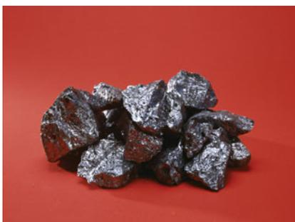
**▲ FIGURE 7.18** Elemental silicon. Although it looks metallic, silicon, a metalloid, is brittle and a poor thermal and electrical conductor.
