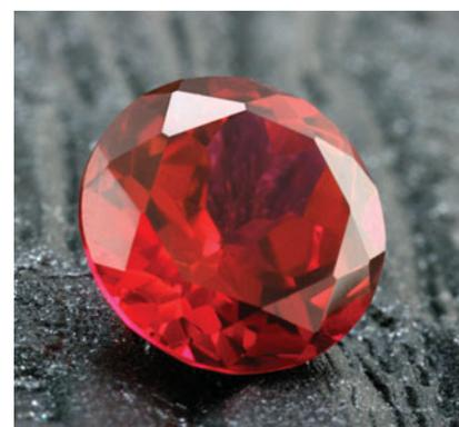
$\blacktriangleright$  FIGURE 12.25 Brittleness and faceting in ionic crystals. (a) When a shear stress is applied to an ionic solid, the crystal separates along a plane of atoms as shown here. (b) This property of ionic crystals is used to facet gemstones, such as rubies.
