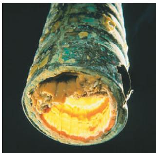
▲ FIGURE 18.22 Scale formation. The interior of this water pipe has been coated with  $\text{CaCO}_3$  and other insoluble salts deposited from hard water.
