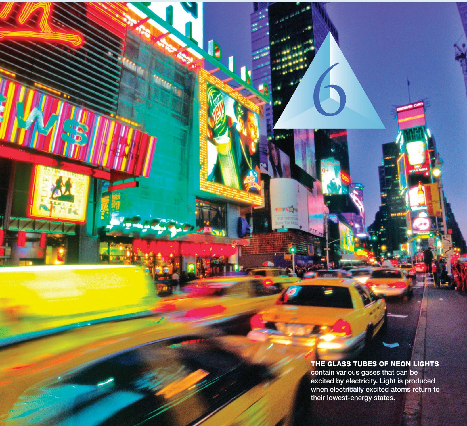
**THE GLASS TUBES OF NEON LIGHTS** contain various gases that can be excited by electricity. Light is produced when electrically excited atoms return to their lowest-energy states.
