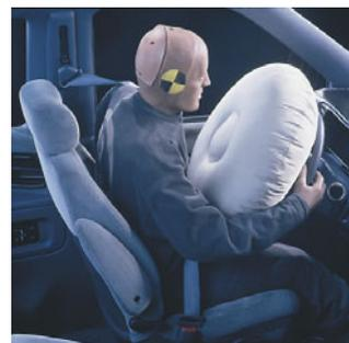
▲ **FIGURE 3.7** Decomposition of sodium azide,  $\text{NaN}_3(s)$ , is used to inflate automobile air bags.
