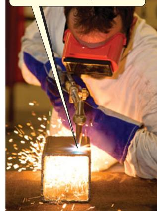
▲ **FIGURE 22.13** Welding with an oxyacetylene torch.
